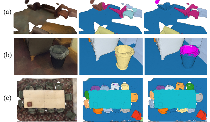
Figure 7: Failure modes of the proposed method. (a) Partial scanning prevents the pose proposal stage from generating plausible poses. (b) Small objects contribute little to the coverage term. If such objects undergo significant motion our algorithm might miss them. (c) When similar, partially scanned objects are considered, our method might not produce the correct permutation.
