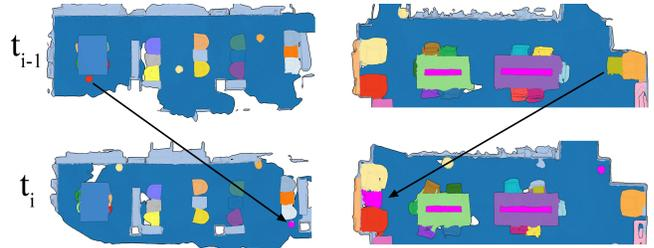
Figure 7: When small objects, like trash bin or coffee table move significantly, our method may not estimate correct instance labels.
