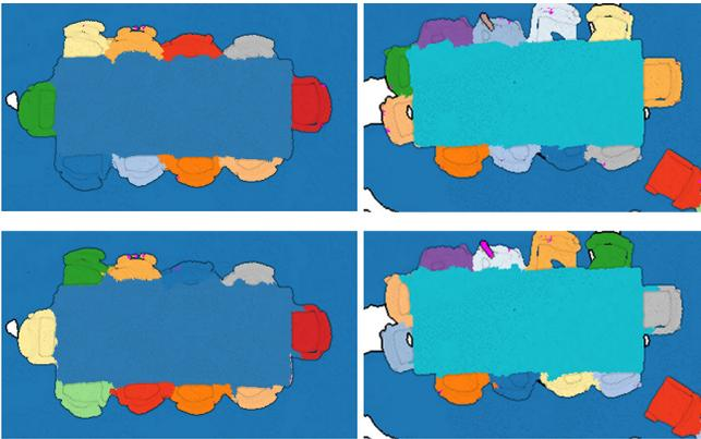
Figure 9: Top - ground truth segmentation. Bottom - predicted segmentation. For sets of visually similar objects our method might produce incorrect permutations of identity assignments.
