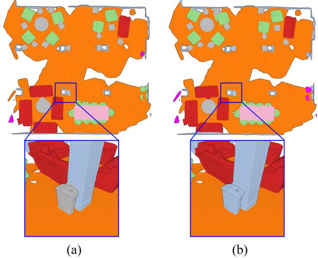
Figure 6: (a) Ground truth segmentation. (b) Semantic label prediction. The lack of trash bins in previous timesteps causes our method to mislabel the trashbin as a part of the column.
